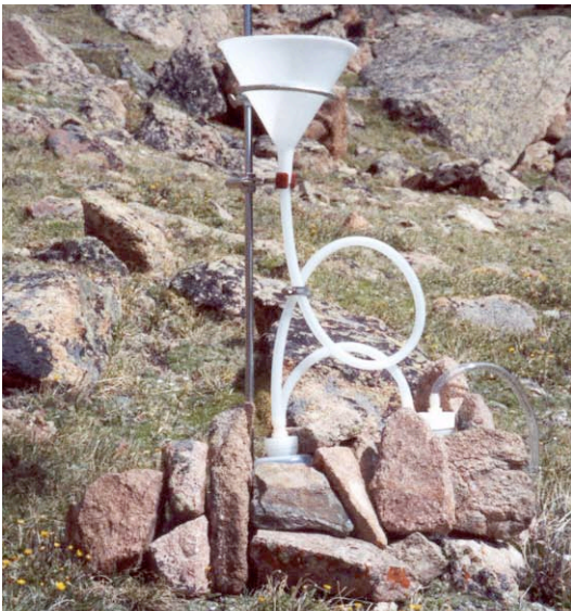
Fig. 2. Hubbard-Brooke rain collector, Middle Mountain, Wyoming, 2001.
